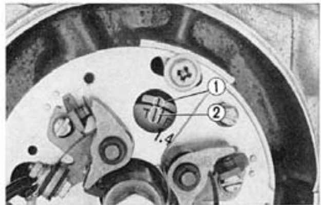
Fig. 3-39 ① Index mark ② "T" mark
