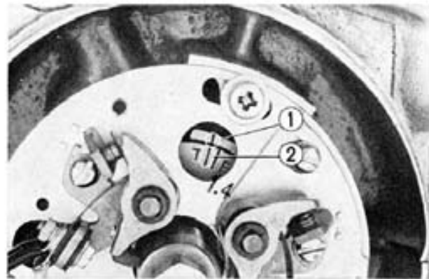
Fig. 3-56 ① Index mark ② "T" mark
